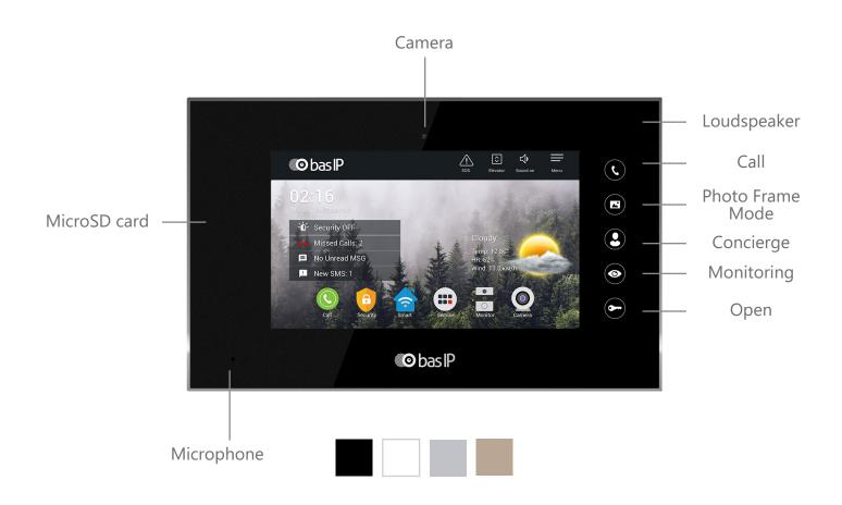
Cloud or Stand-Alone SIP Integrated with Access Control & VMS 7" TFT Screen Customizable "Do Not Disturb" Connect up to 32 IP Cameras Full Duplex Audio PoE or 12VDC Input Power Record Audio/Video with Optional SD Card Ability to Install 3rd Part Applications
